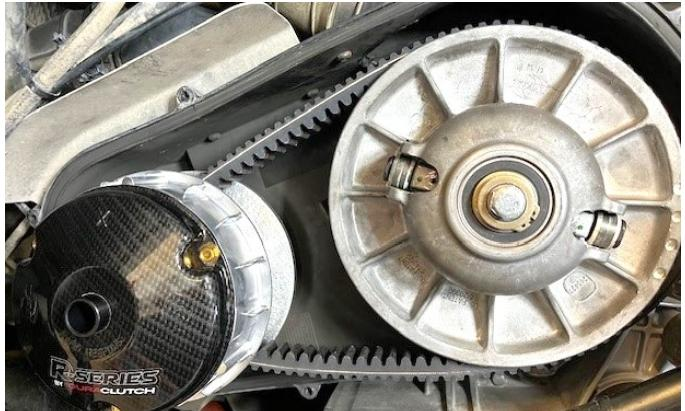
8. Install DURA CLUTCH Primary with hardware provided as shown below. **VERY IMPORTANT -Torque bolt to 60 ft-lbs.**
