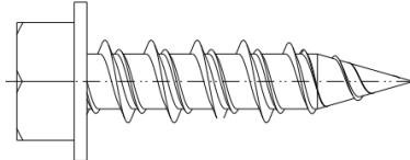
Torque spec: 50 in-lbs (4 ft-lbs). This is like a screwdriver torque. Use a hand wrench or a clutch screw gun at a very low setting.
