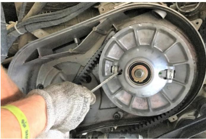
7. Slide belt into primary clutch, then install on post.
