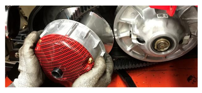
8. Set belt tension. Place transmission in Park and make sure machine is turned off. Rotate secondary by hand to seat belt in secondary clutch until belt tension is tight.
