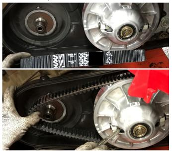
7. Slide belt into DURACLUTCH DCR Primary clutch then install on post. Use stock primary hardware removed in step 5. Tighten bolt to 47 ft-lbs.
