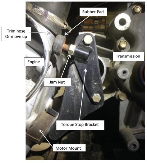
MODEL OF TORQUE STOP INSTALLATION WITH CLUTCH HOUSING BACK REMOVED
