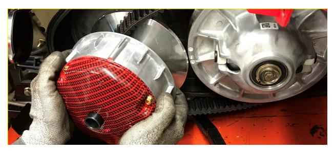
7. Tighten stock primary bolt to **60 ft-lbs**. **VERY IMPORTANT**- Over tightening will not allow clutch to operate properly and cause damage and failure of the clutch.
