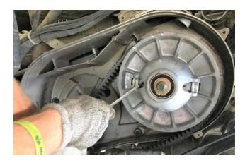
6. Slide belt into primary clutch, then install on post. Use primary hardware removed in step 3.
