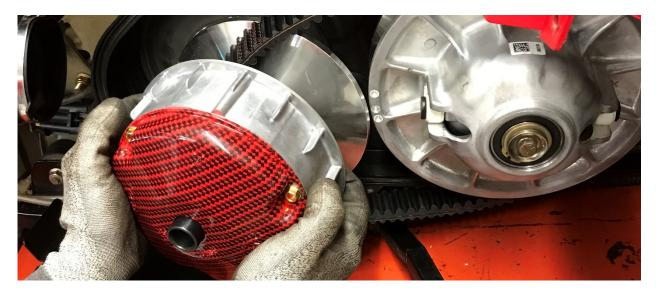
8. Set belt tension. Place transmission in Park and make sure machine is turned off. Rotate secondary by hand to seat belt in secondary clutch until belt tension is tight.
