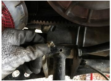
2. Remove stock secondary clutch. Install qty (2) 90-061- 0.060 shim washer and qty (1) 90-060- 0.036 shim washer on the spline shoulder. =.156 of total spacing. Install the DCR Secondary.
