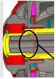
3. Install the M10X1.25X65 provided with kit as shown below. Use the washer that was under the screw head. Place Blue Loctite provided on the secondary screw threads. Tighten screw to 45 ft-lbs.
