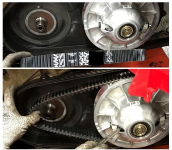
7. Slide belt into DURACLUTCH DCR Primary clutch then install on post. Use stock primary hardware removed in step 5. Tighten bolt to 47 ft-lbs.
