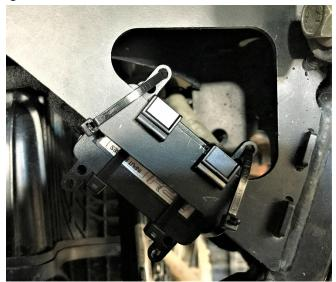
18. Disconnect speed sensor on transmission. Connect end from dongle to transmission. Connect wire removed from transmission into other end of dongle. Make sure Dongle does not interfere with any moving components, such as suspension or shifting assembly. Use remaining cable ties to secure wires as necessary and clip excess tie ends.
