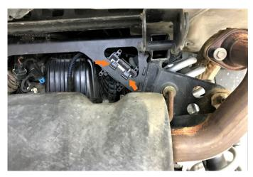
17. Take two 8-inch cable ties and feed thru tab on top of dongle housing and around the frame and tighten
