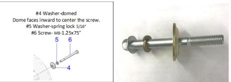
6. Remove Primary clutch bolt. Remove the Polaris primary outer movable sheave assembly. Pull off by hand holding the central shaft in place with your thumb. Move around the clutch, with a pulling and rocking motion.
