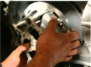
7. Pull the Polaris primary fixed sheave from the engine crankshaft using PN 99-030 puller. Greasing the end of the puller slightly will aid in removal. Do not get grease on any clutch components.
