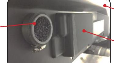
Stock clutch air intake on passenger side door post
